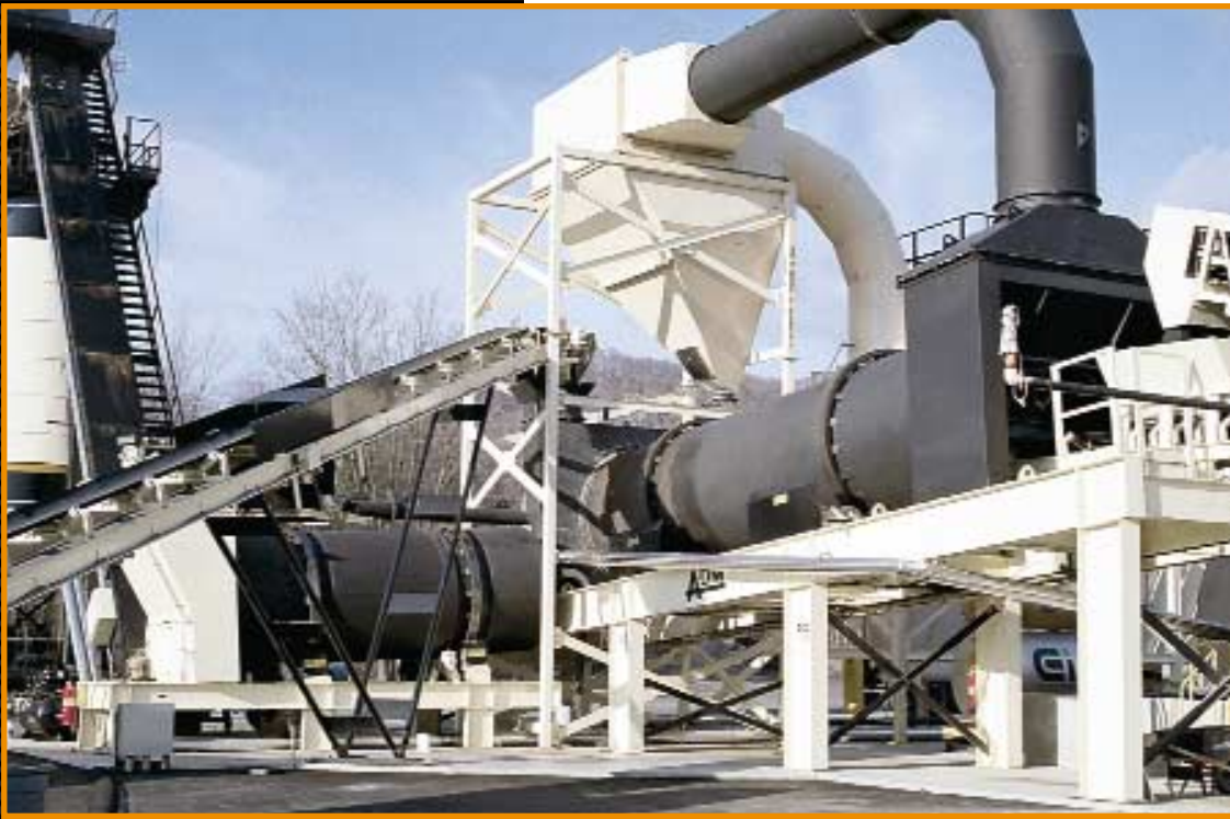
Separate drying and mixing drums give Tarheel Paving's ADM plant long drying times and clean operation.
